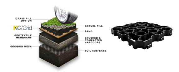
KC/Grid Ground Reinforcement System is manufactured in the UK from 100% recycled plastic. Suitable for a variety of applications including both domestic and commercial car parking, embankment stabilisation, golf courses, pathways and many more. KC/Grid is an environmental alternative to tarmac and concrete.
